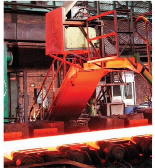
Steel Hot Strip Mill
